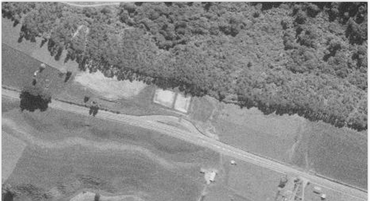
Historic aerial image (1995) showing modification of site including removal of direct road access through construction of layby for Stock Effluent Disposal site (pale rectangles in centre). Drovers' Trough is visible to immediate right of layby.
