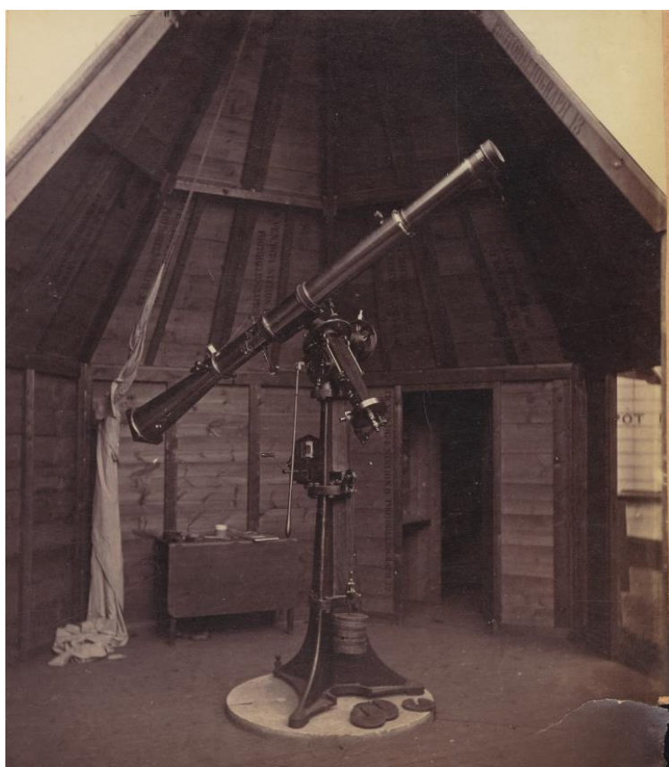
Figure 7 Dallmeyer photoheliograph, RGO 6/276: 20. This image shows the interior of Station D photoheliograph enclosure during trials in Greenwich. The central door leads to the adjacent darkroom. The stencil on the timber interior of the hut states 'Station D' which shows this was destined for New Zealand. (Copyright Cambridge University Library, Licensed under Creative Commons Attribution – Non-Commercial).
