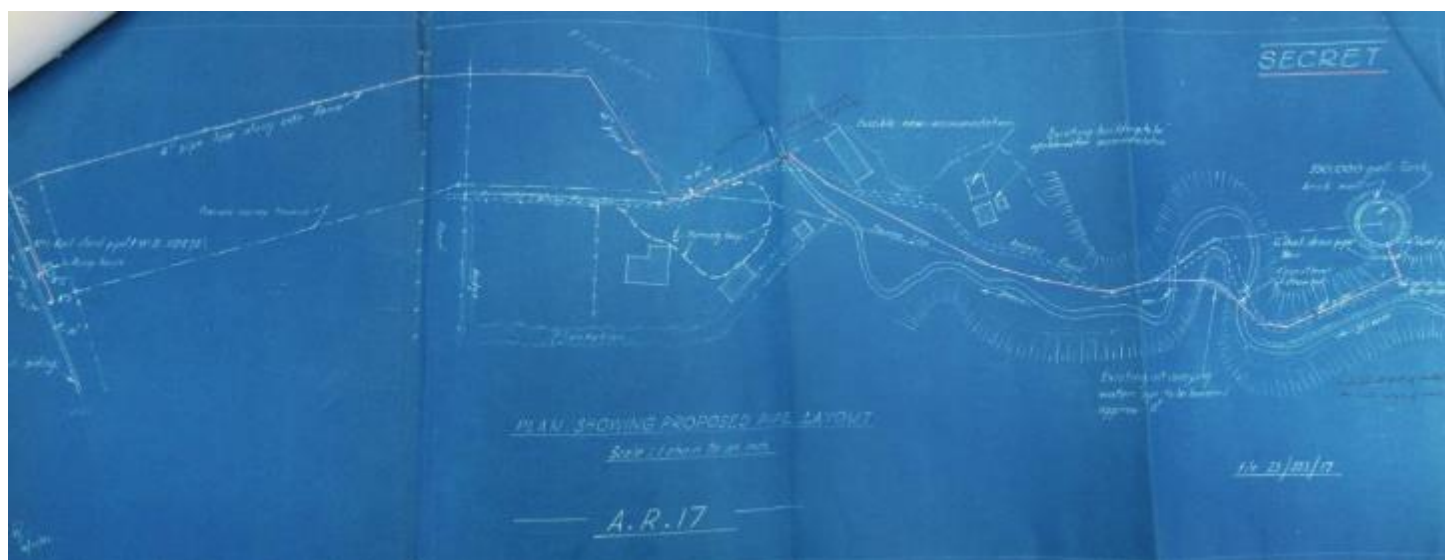
Fig 3: 'Plan showing proposed pipe layout: AR17', PWD 114701, dated 10/11/42. Copy on file 'Defence Works and Buildings – Air Department Royal New Zealand Air Force [RNZAF] bulk fuel storage – Site AR17 – Paekakariki 1942-1942'. Item ID R21064922, box 796, file 23/553/17, Public Works Department (ACHL), Archives New Zealand.
