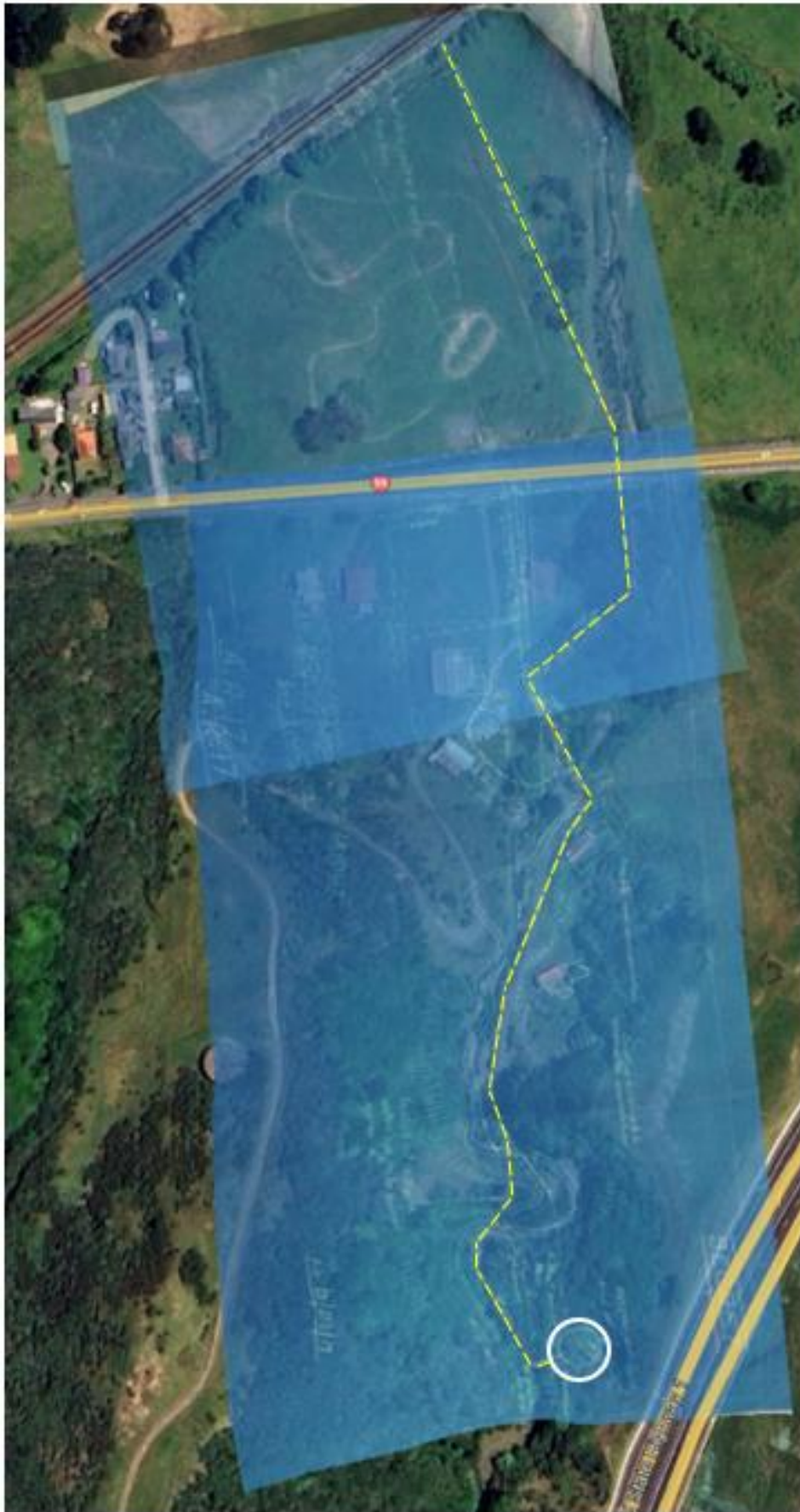
Fig 4: 'Plan showing proposed pipe layout: AR17', PWD 114701, roughly overlaid on modern Google Earth aerial to map possible pipeline position.
